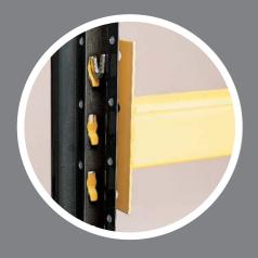
Each beam is supplied complete with a pair of steel Safety Locking Pins. When located they ensure the beam is correctly positioned and help prevent the beam being dislodged during use.
